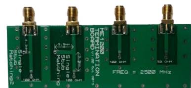
Termination board tuned at 2500MHz:
